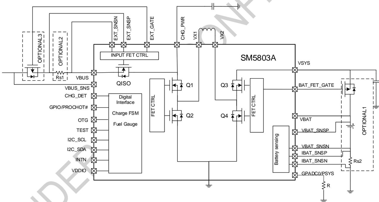
OPTIONAL1 = Required when connecting to a battery else not needed
